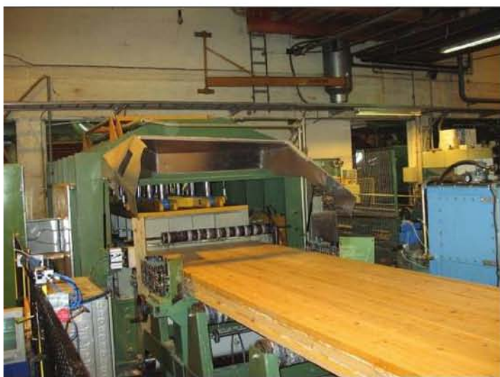
This CLT manufacturing plant uses a radio-frequency press.
